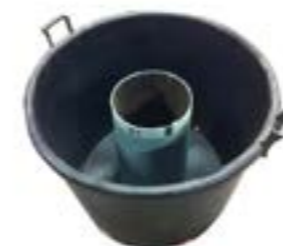
Base in weighted bucket
